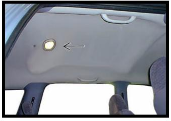
1. Remove and retain O.E. dome light by gently prying downward on rear edge of lens then slide frame assembly out. Disconnect wiring and lay dome light in a safe place. See Fig. 1.
